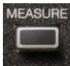
Press the front panel Measure button to access the Measure menu and turn the measurement parameters on. Press it again to turn the parameters off.
