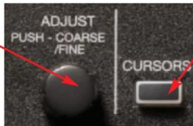
Press to turn cursors on, toggle through the cursor types, and then turn the cursors off. Choose between Time, Amplitude, Time & Amplitude, and Value at Cursor.
