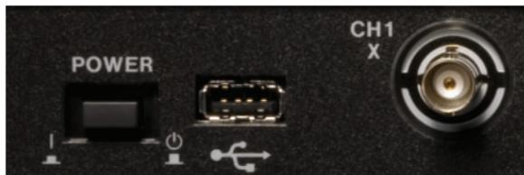
Connect a USB memory device to the front panel USB port.
