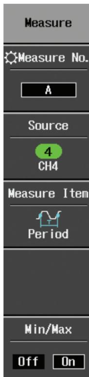
Up to 4 measurements can be displayed at a time, select between measurement lines A, B, C, D.
