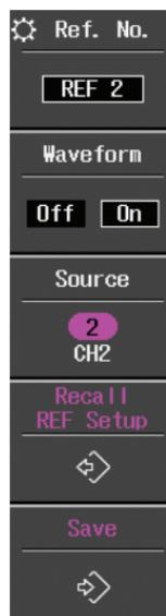
Select between 5 different Reference waveforms.
