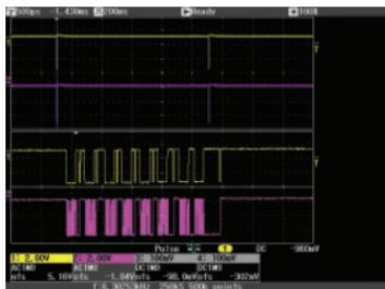
After Quick Zoom is pressed the zoom traces are displayed in a separate grid.
