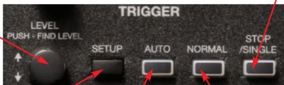
Press to open the trigger setup menu.
